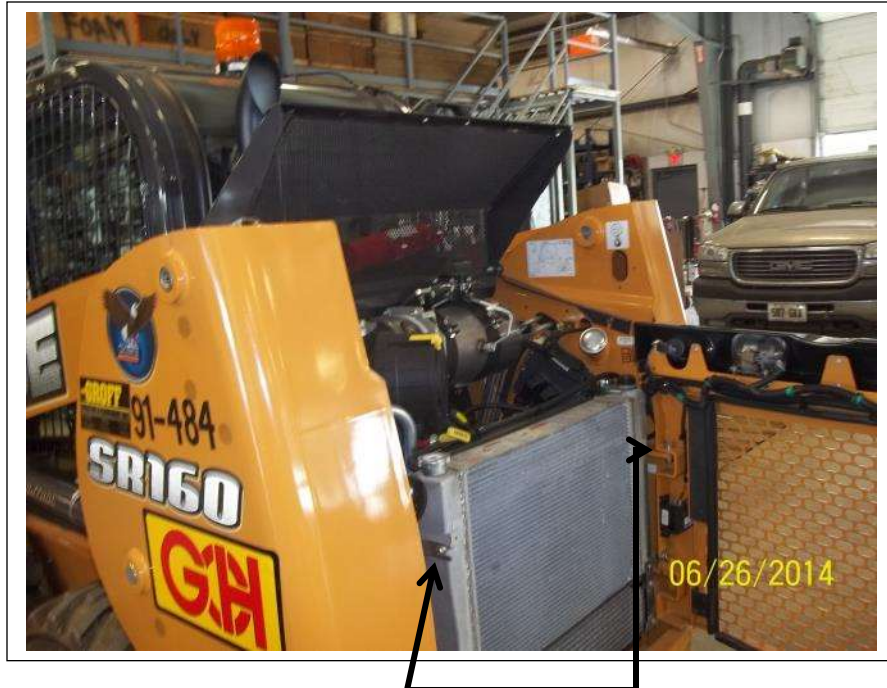
Loosen two bolts (one at each side of rad) Allows rad to tilt toward yourself. Detach top and bottom rad hoses
