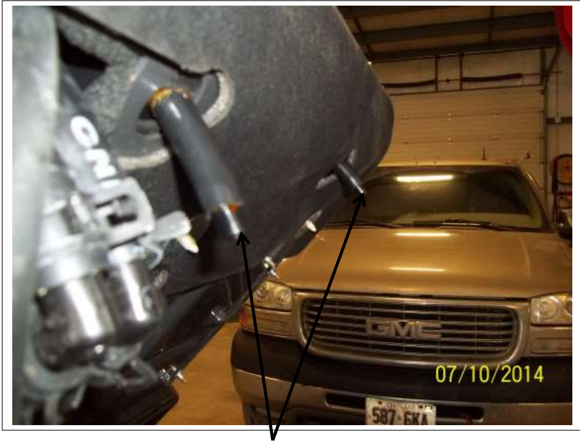
Drain tube restrictors glued into the drain tube.
