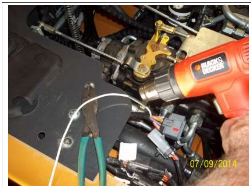
Follow simple wiring diagram to determine which 30" lead connects to # 237A Shrink wrap fitting after proper crimp
