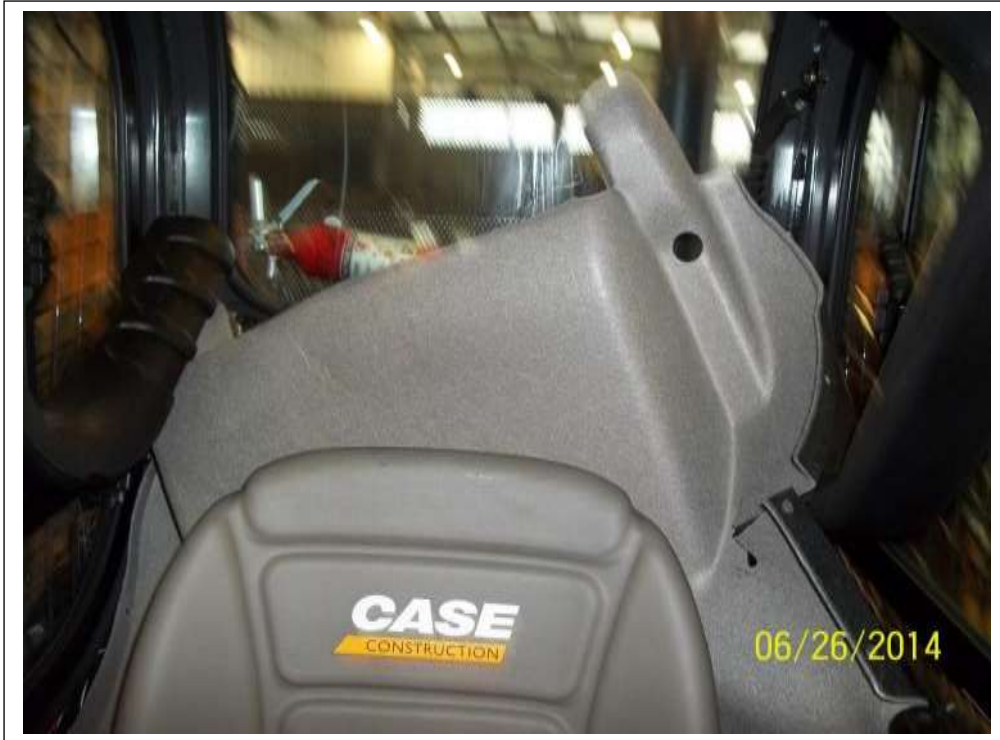
Remove cover and lift over seat to gain access to the heater box.
