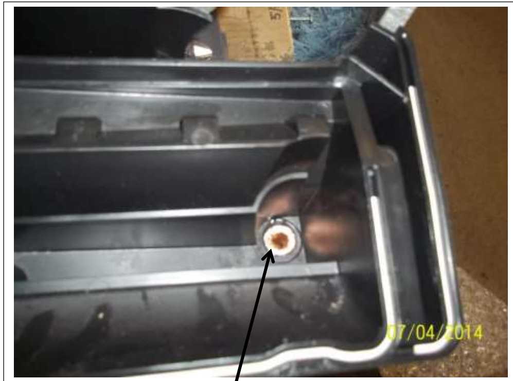
Glue in copper drain tube extensions. 2 required.
