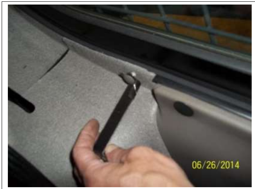
A simple tool could be made which helps remove the button clips
