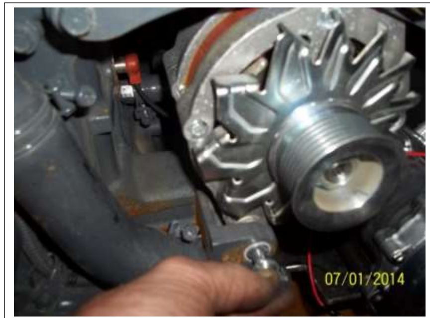
Loosen top alternator tightener and belt prior to removing the lower fastener bolt for the alternator.
