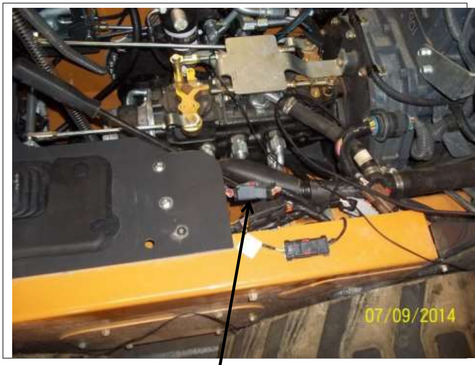
With the cab tilted up again, find a large bundle of wires along the left side with a number of quick disconnects. Identify a larger multi pin grey disconnect and pull it apart from the rest.
