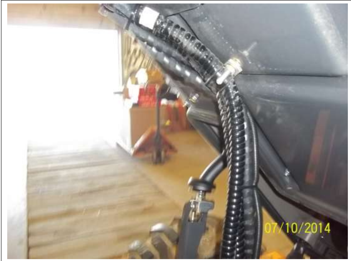
A/C lines fastened along with the heater hoses. Allow sufficient slack ( similar to the heater hoses) to be able to open and closed the cab
