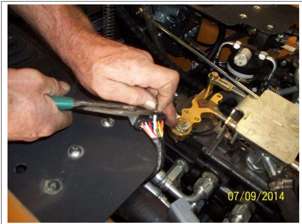
Pull that white wire out of the socket or cut it very close to the socket
